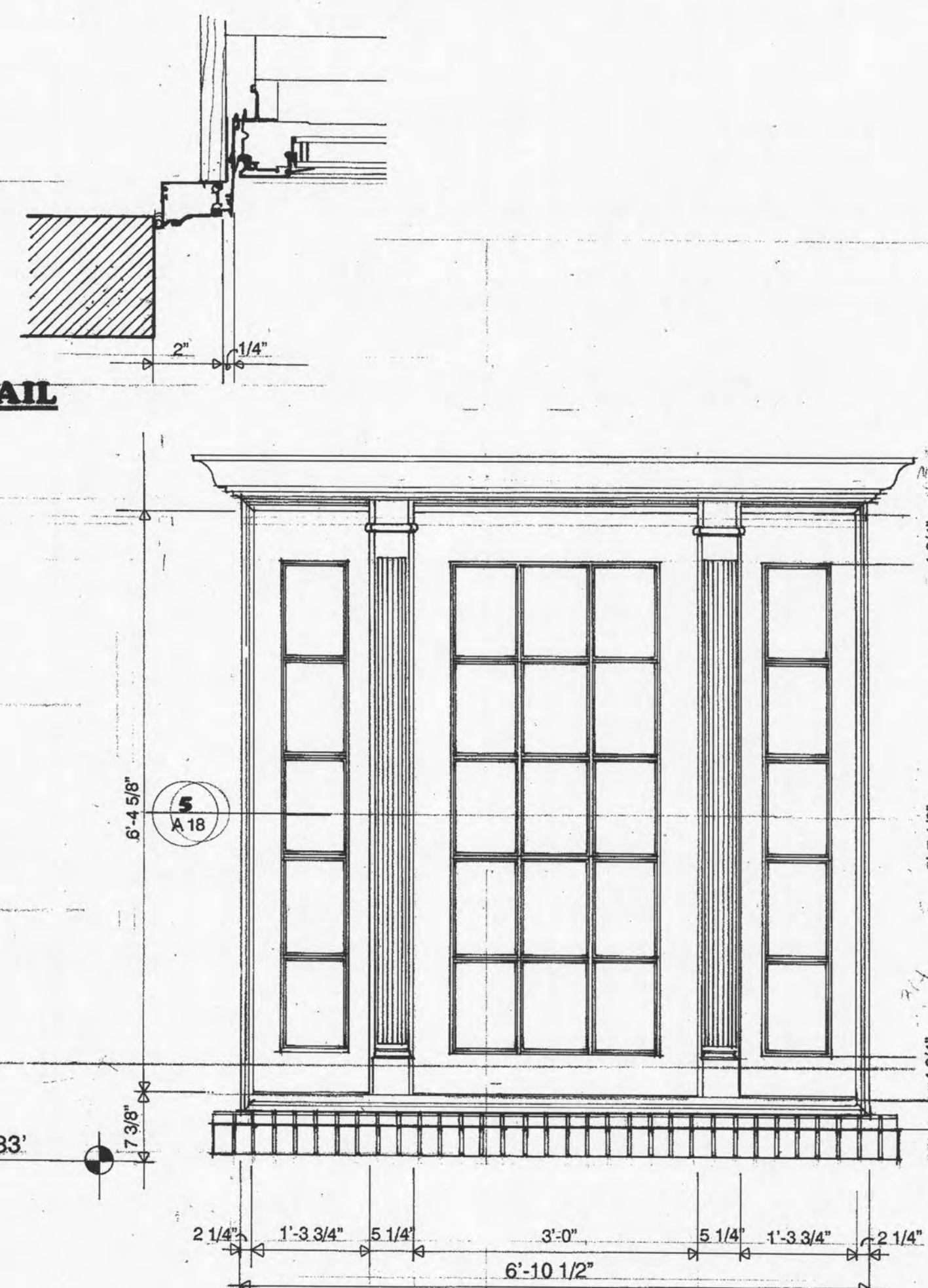
3 WINDOW ELEVATION SCALE: 3/4" = 1'-0" (LEVEL III)
